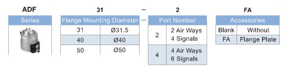
Order Example: Flange Mounting Diameter: Ø40; Port no.: 2 air ways; 4 electrical signals. Order Code: ADF40-2
