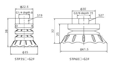
Note: The dimensional tolerance conforms to GBT3672.1 -2002-1 M3 rubber product dimensional tolerance standard
